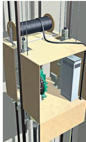
***The KONE JumpLift** is a self-climbing elevator that uses the building's permanent hoist way for construction time use. The Jumplift is available before the permanent machine room is ready. It has a temporary machine room that moves upward ('jumps') as the construction work progresses. Each jump can be carried out at times that suit other construction activities.*
